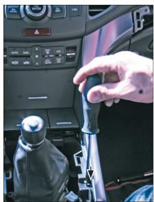
6. Remove screws of inner side panels beside gear lever
