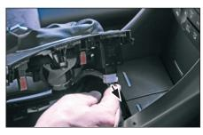
2. Turn panel aside and remove plugs carefully (see arrow)
