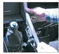
Remove screws of air condition control unit
