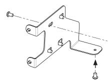
21. Fix Double DIN navigation to vehicle dashboard from underneath (see arrow)
