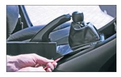
1. Unclip panel under gear lever
