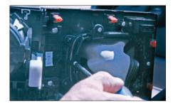
3. Remove screws around gear lever in order to remove panel
