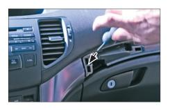
Remove screws of inner side panels
