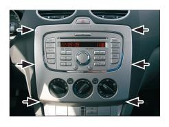
Unclip the frame surrounding the OEM-Radio and remove it
