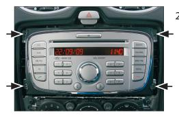
Remove the four screwsRemove the OEM-Radio
