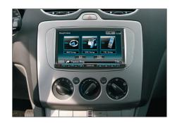
. Push the head unit with the mounted metal brackets into the metal frame, until it snaps in
