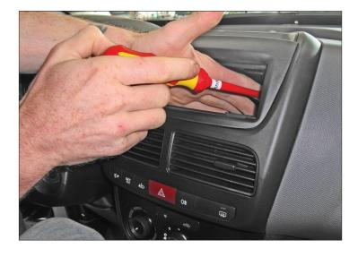
2. Remove 2 screws (left and right)
