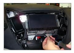
Mount mounting frames to double DIN head unit
