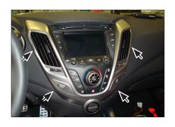
Unclip OEM panel with air vents (see arrows)
