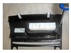
4. Remove hazard light switch and display from OEM bezel
