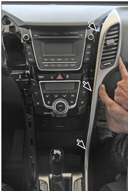
3. Remove side panels with air vents at left and right side (see arrows)
