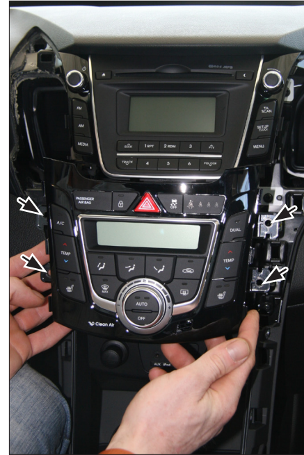
4. Remove screws (see arrows) Remove control unit
