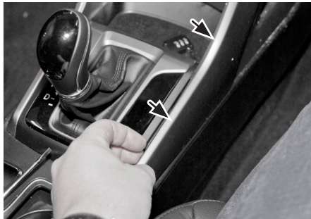
2. OEM side panels need to be removed. Start at this position (see arrows)
