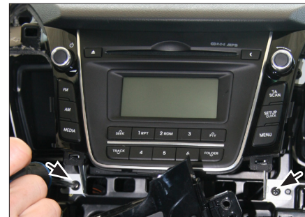
5. Remove screws (see arrows)
