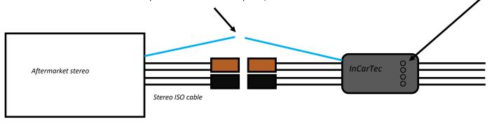
If the new stereo does not have a loose remote output wire, tap the amp turn on wire onto the blue antenna turn on wire that's already wired in the ISO lead.
