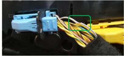
the patch lead to the interface on the radio replacement harness and the new radio.
