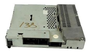
the new radio. The Brown Fakra is for the rear view camera, the beige Fakra is for the Venture Cam. If the radio being fitted only has one input an additional video source switcher may be required.
