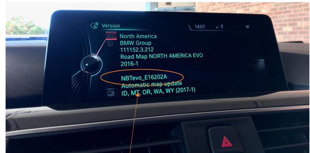
If NBTevo_XXXXX appears on the version then it is a NBT EVO
