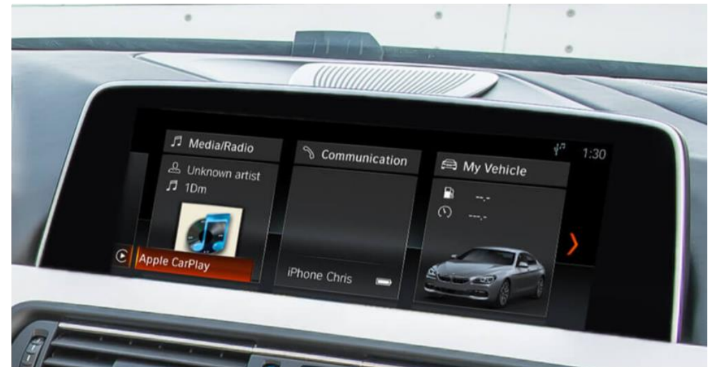
The ID6 main screen consists of a series of horizontal tiles on a grey and black background, with a red/orange gradient highlighting the selected feature.
