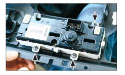
Remove pocket above radio frame (unplug all connectors carefully)
