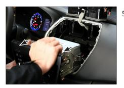
Disconnect all cables and remove OEM head unit
