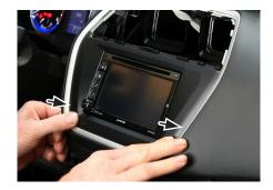
Connect all required circuit points and push Double-DIN head unit into dashboard
