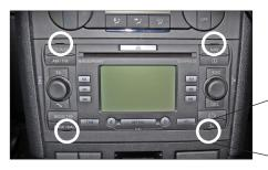
1. Insert four Ford Mondeo radio release keys in the OEM head unit.
