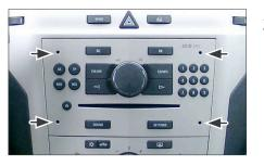
2. Put the radio release keys in the holes of OEM radio (see arrows)
