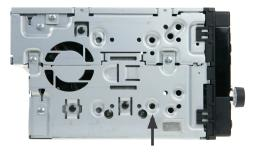
Mount the metal brackets to double DIN head unit
