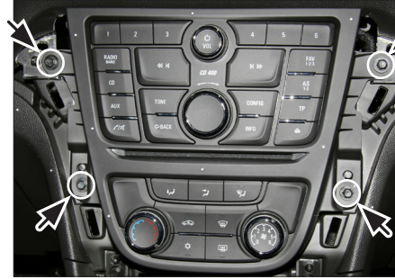
5. Remove screws of OEM head unit
