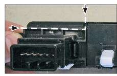
Cut out fin on both sides (see arrows) 8. Place the Hyundai OEM panel on the dash board
