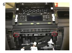
6 Unscrew and save the 2 screws circled in red. Remove the keys panel. Disconnect and remove the radio from the radio tunnel
