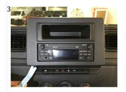
3 Remove the OEM facia plate as shown in the picture.
