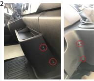
2 Unscrew and save the 4 screws circled in Red and remove the plastic panel.
