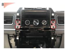
8 Connect all cables, verify the proper functioning of the system and install the radio in the radio tunnel by tightening the screws save previously.
