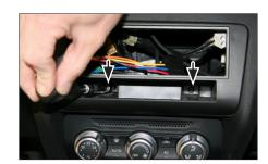
6. Fix facia plate with 2 OEM screws (removed in step 3)
