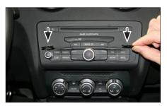
2. Use special radio release keys to remove head unit (see arrows)
