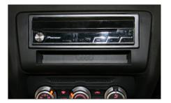
8. Connect all required circuit points Push head unit into facia plate
