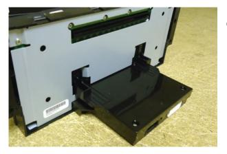
6. Undo the screws holding the control module to the front button panel.
