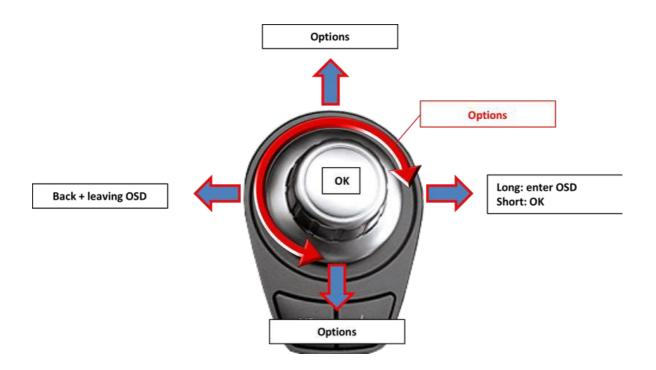
**Note:** If the interface is selected as active video source then the OSD menu is activated via iDrive button "**OK**" (press and hold) + "**iDrive-right**". In this OSD menu only image adjustments can be made.
