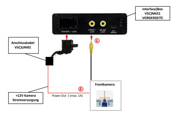
Connect the video RCA of the after-market front camera to the female RCA connector "FRONT CAM" of the interface box V5C-M631.
