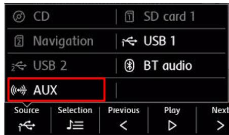
**NOTE!** Make sure switch to "AUX" mode on original car stereo for audio transmission before using the CarPlay integration.
