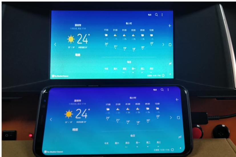
Connect Android smartphone/iPhone with USB cable, and then enter “MirrorLink” for screen mirroring.
