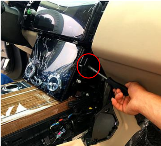
4. Take out the two sides screws of OEM below screen
