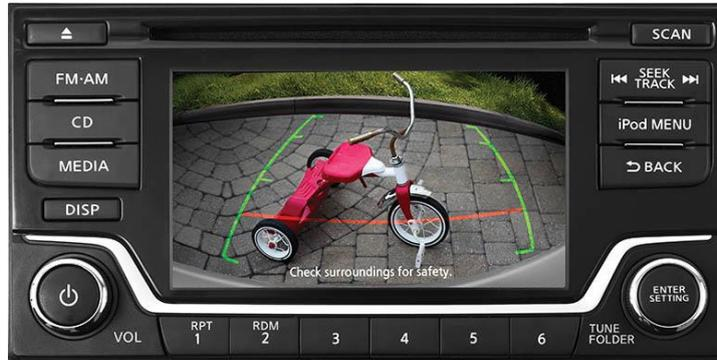
Depending on the cameras view angle and the place it is installed, the parking lines may not be accurate and will then need to be adjusted in the diagnostic menu of the car radio.
