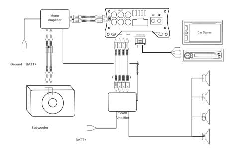
Example 2 shows the DSP amplifier used as a signal processor to supply audio to additional amplifiers
