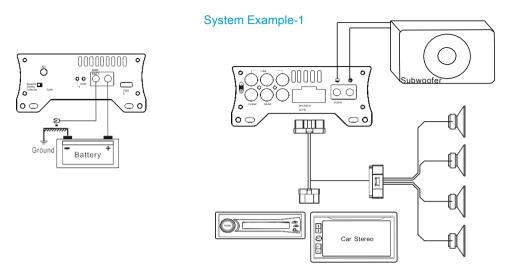
Example 1 shows the DSP amplifier used to drive the speakers in the car plus a passive subwoofer
