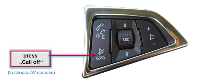
A press of the steering wheel's CALL OFF-button switches the input from factory mode to the inserted video sources. If, by dip switch setting, all inputs are enabled, the order is the following:
