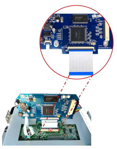
Connect the daughter PCB's pre-assembeled 66pin ribbon cable "IN PCB" to the previously become free ribbon cable base of the monitor mainboard (heed the following warning notes!).
