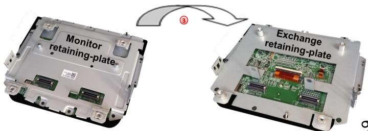
Remove the Original monitor retaining plate and replace it with the exchange retaining-plate by using the original screws. Page
