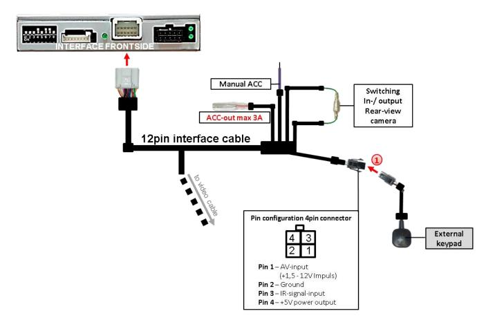
Onnect the keypad's female 4pin connector to the video-interface's male 4pin connector.
