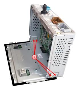
2 Turn out the 4 screws of the monitor retaining plate, after carefully unklipping the 66pin and the 9pin ribbon cables.
