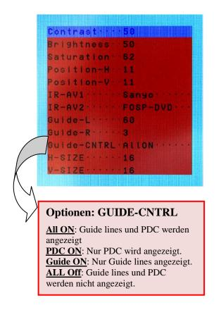
**Note:** If the CAN-box does not support the vehicle's CAN, the guide-lines cannot be used.
