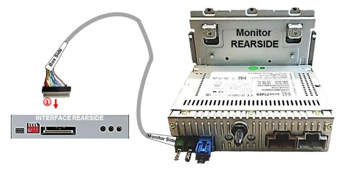
Connect the female 20pin LVDS connector of the LVDS cable which is led out of the head unit, to the male 20pin connector of the video interface.
