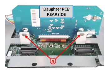
After connecting the ribbon cables, the daughter PCB has to be fixed with its rearside at the exchange retaining plate by using the enclosed 2 shorter screws.
