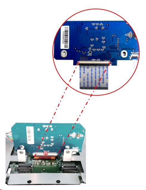
Connect and clip in the 66pin short, kopper-coloured ribbon cable which is led out from the monitor and connect it to the free ribbon cable base "OUT-PNL" of the daughter PCB's rearside (heed the following warning notes!).
