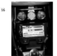
Finally, clip the fascia panel into place and reinstall all components in the reverse order of disassembly to complete your installation.
