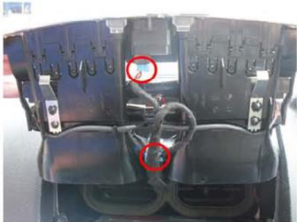
Remove airvents and disconnect the two Blue connectors from underneath vents.
