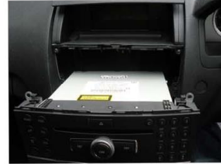
Guide the head unit from the dash. There are runners as shown bellow.
