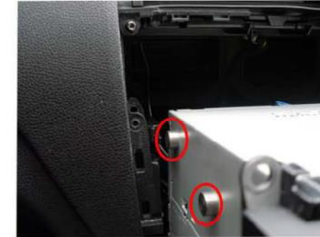
Guide the head unit from the dash. There are runners as shown bellow.
