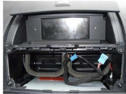
Remove airvents and disconnect the two Blue connectors from underneath vents.
