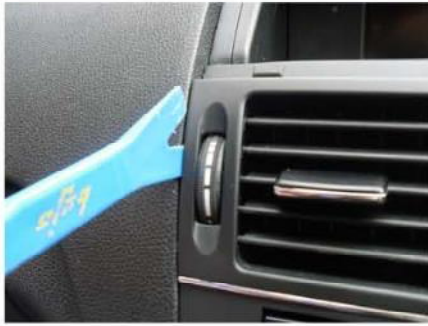
Remove airvents and disconnect the two Blue connectors from underneath vents.
