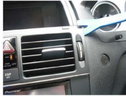
Remove airvents and disconnect the two Blue connectors from underneath vents.
