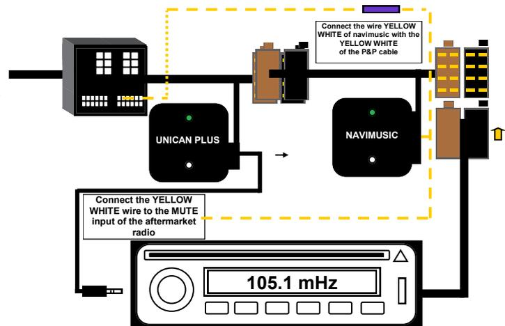
**This interface will automatically turn on the navigation unit. You can manually turn on the navigation unit by pressing and holding the mute button on the steering wheel.**
