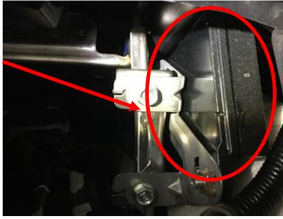
Connect the loose green wire from the 29-679 to the 2<sup>nd</sup> Pin from the end (**blue or green wire**) as shown in the image.
