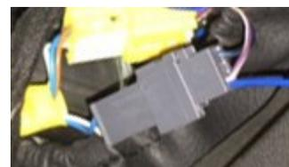
Identify the steering wheel control signal wire under the steering column. This will be a wire that rests at 4.5V on a 2 or 3 way connector. This voltage will fluctuate when buttons are pressed on the steering wheel.
