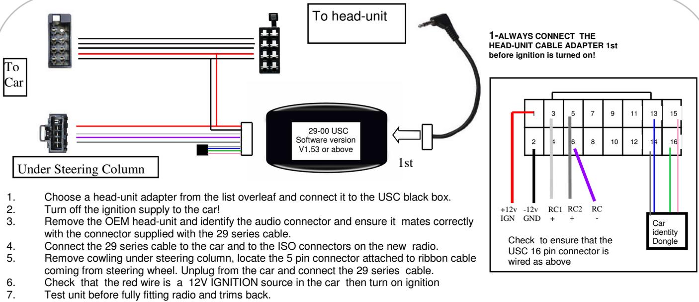
**If Problems:** Check that correct adapter has been used and links are in the correct place. Always disconnect from the power supply if you change the head-unit adapter lead. Check that Red wire is 12V ignition and not Permanent power. Check that head-unit is earthed and black wire is earth. Check all connections are the same as the wiring diagram shown here
