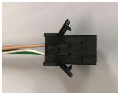
3. Using a small pick, **carefully** lift the retaining tabs at the front of the connector. With it lifted slightly, pull the wire to release the terminal. **Be careful not to damage or snap the retaining tabs or the new terminal will be loose.** Insulate and disregard the terminals on the original wiring loom.
