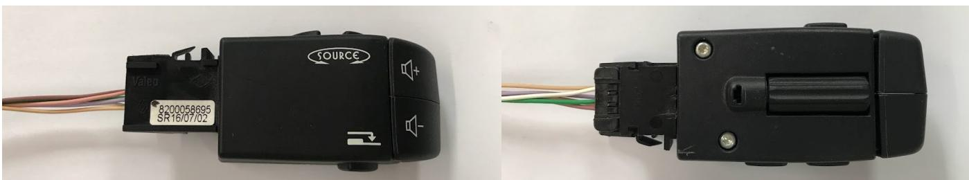
2. This is the black wiring connector that is required to fit the 29-608-LOOM. It needs to be removed from the terminals on the original wiring loom. Begin by using a small pick or flat blade screw driver to open the retaining clips in the middle of the connector.
