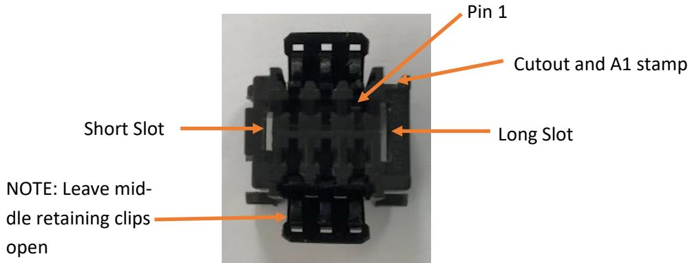
2. Flip the connector over to view the back, ready to insert the terminals from the 29-608-LOOM. Pin 1 (next to the cutout and A1 stamp) should now be top left.
