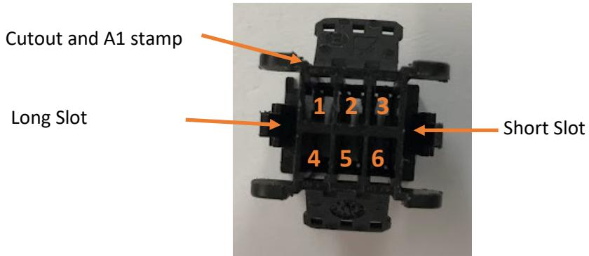
3. Insert the terminals of the 29-608-LOOM into the connector as per the following list and diagram, making sure they clip into place on the retaining tabs at the front of the connector. When they are all in place, push the retaining clips in the middle of the connector to fully lock the new terminals in place.
