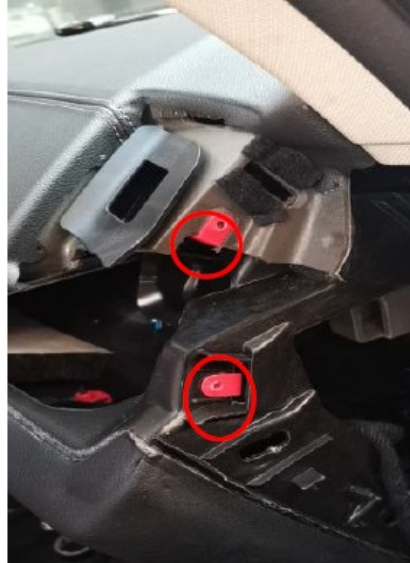
9. Use a panel tool to tilt down the fixed bezels on the display and remove the screws on both sides
