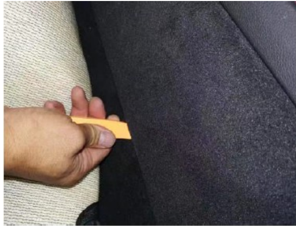
2. Use a panel tool to lift the left and right interior away.
