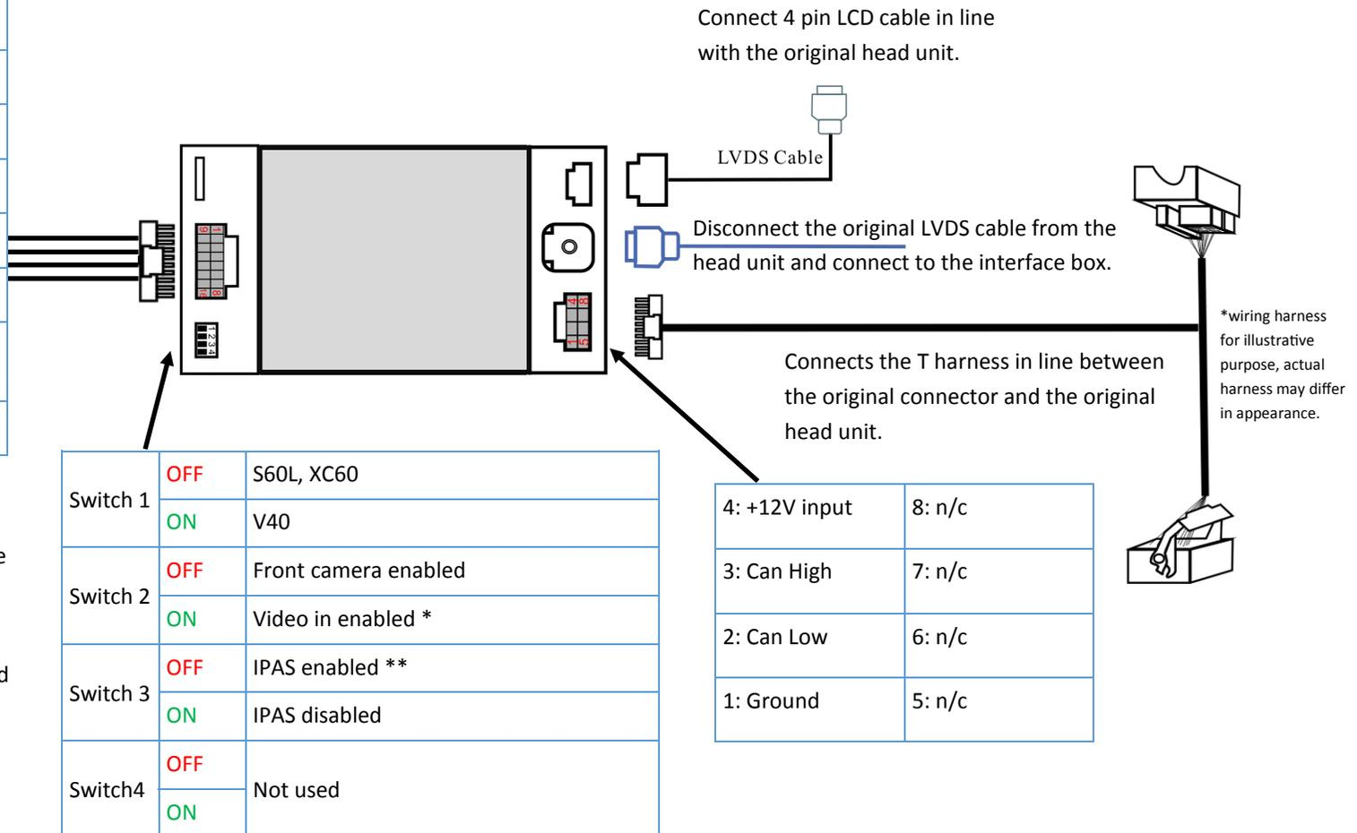
The switches need to be set before the interface is powered. If the switches need to be changed the interface will need to be disconnected from the power to reset.
