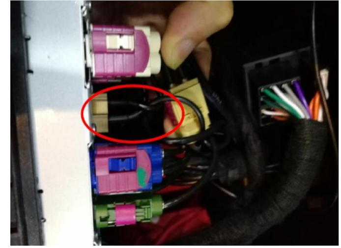
Unplug the LVDS Connector and connect the new LVDS IN connector to the head unit. Connect the original LVDS connector to the LVDS OUT connector from the in-
