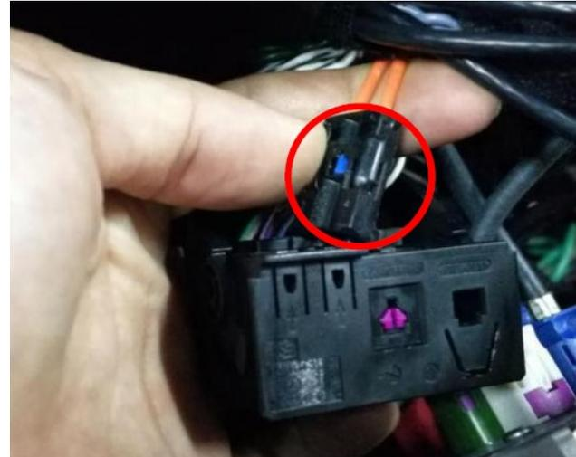
Remove the OEM Quadlock and move the Fiber-optic plug to the new quadlock on the interface
