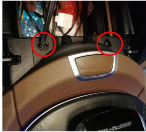
Remove the two screws and lift away the plastic fascia cover
