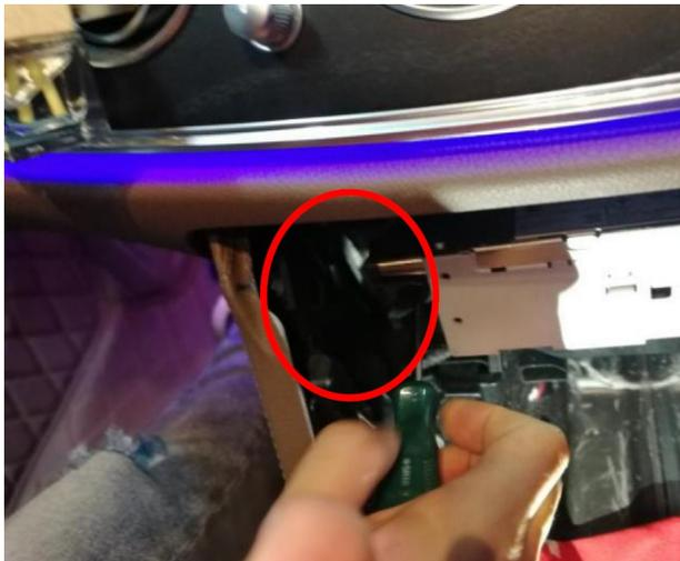
Remove the screws holding the head unit in place and pull away the radio from the dash
