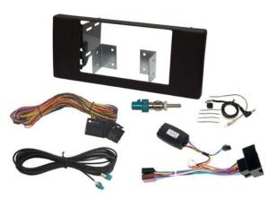
Complete fitting kit to install a double DIN head unit and retain the original steering wheel controls in a **BMW X5 E53**
