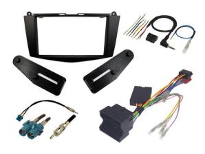
Complete fitting kit to change the original radio in Mercedes vehicles for a double din after market unit. FOR VEHICLES WITHOUT SWITCHES BELOW THE RADIO.
