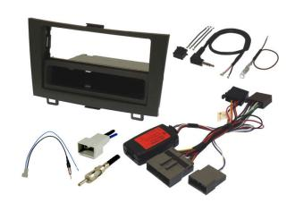
Complete fitting kit to change the original radio in a 2007-2011 Honda CR-V for a single or double din after market unit.
