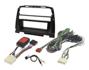
Complete fitting kit to install an aftermarket single din head unit into a 2000-2005 model Jaguar XK8 convertible with original premium audio.
